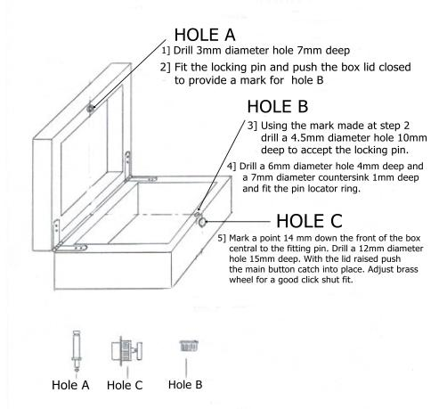
For best results use a drill press. Minimum wall thickness 15mm
